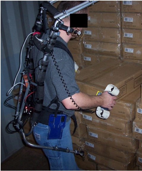
Figure 1. Moment monitor on worker.
