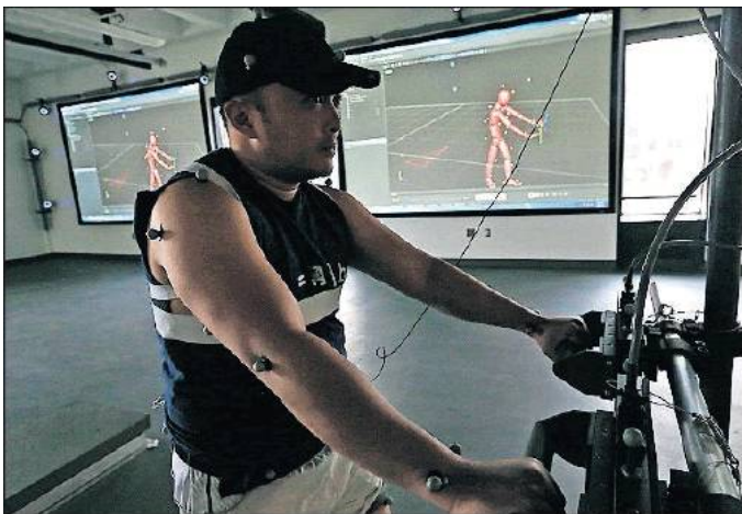
Doctoral student Peter Le pushes a beam around a room while being tracked by sensors.
